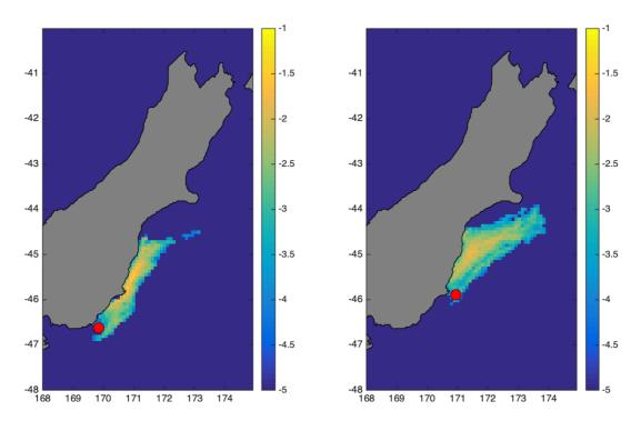
Figure 1: Example physical oceanographic model output used to aid connectivity estimates. Colour is the Log distribution of the probability that a particle lands in a 10 km x 10 km grid around the South Island, 10 days after release. Release locations Long Point (left panel) and Otago Peninsula (right panel) are denoted by the red circles.
